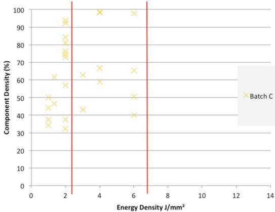
Batch C displays significant component density variation. In some circumstances good densities have been achieved, however, it demonstrates clear sensitivity to changes in process parameters, producing unreliable results.
