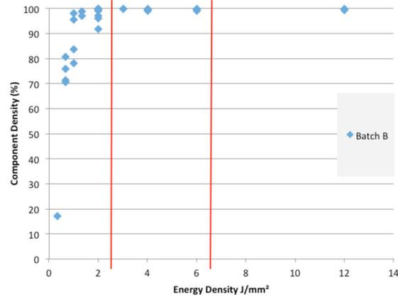
Batch B displays good component density achieved at a wider range of process parameters. This demonstrates that even with some changes to process variables acceptable component density can still be achieved.
