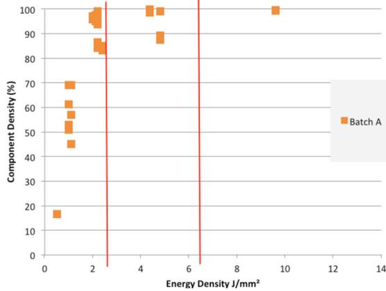
Batch A demonstrates that, as expected, as energy density increases so too does component density. However, it can also be seen that at 2.5 – 6.5 J/mm<sup>2</sup> (indicated by the red lines) both acceptable and unacceptable parts are produced as parameters vary.
