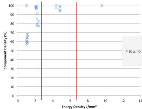
Batch D displays similar results to Batch A - some acceptable densities, but slight changes in process parameters result in poor component density.
